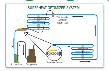
accurate superheat control, thus fully flooding the evaporator. The TXV sensing bulb is secured to the outer sensor tube. To further assist the superheat reading, a groove is formed in the outer tube, of the superheat sensor, to provide additional thermal contact and ensure perfect alignment of the TXV bulb to the suction line.
